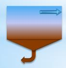
3. In this stage, particles such as silt begin to attach to each other in the flocculation chamber, settle to the bottom, and are removed through the bottom of the sedimentation chamber—further clarifying the water, which flows to the next stage.
